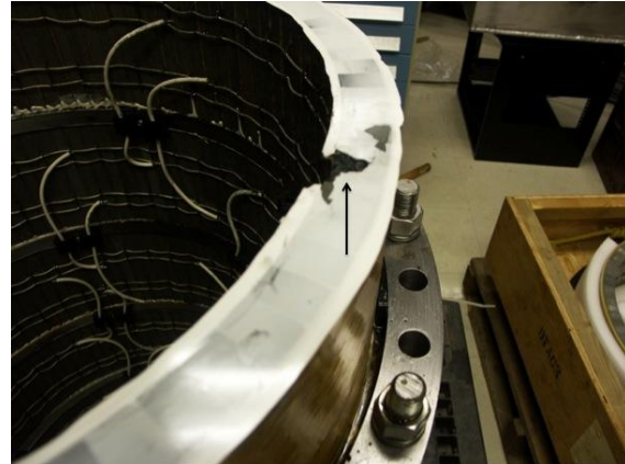
Figure 5. (Left) The weak signals from the accelerometer are shown here for all three accelerometer axes. The direct wave arrives at about 0.033 s. It is not possible to distinguish between the pressure-wave and shear wave on the basis of this signal. (Right) The source of the signal weakness – a transducer ring burned (arrow) from electrical arcing.
