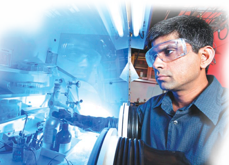
ORNL's Jagjit Nanda assembles a lithium ion battery for performance testing within a controlled environment.
