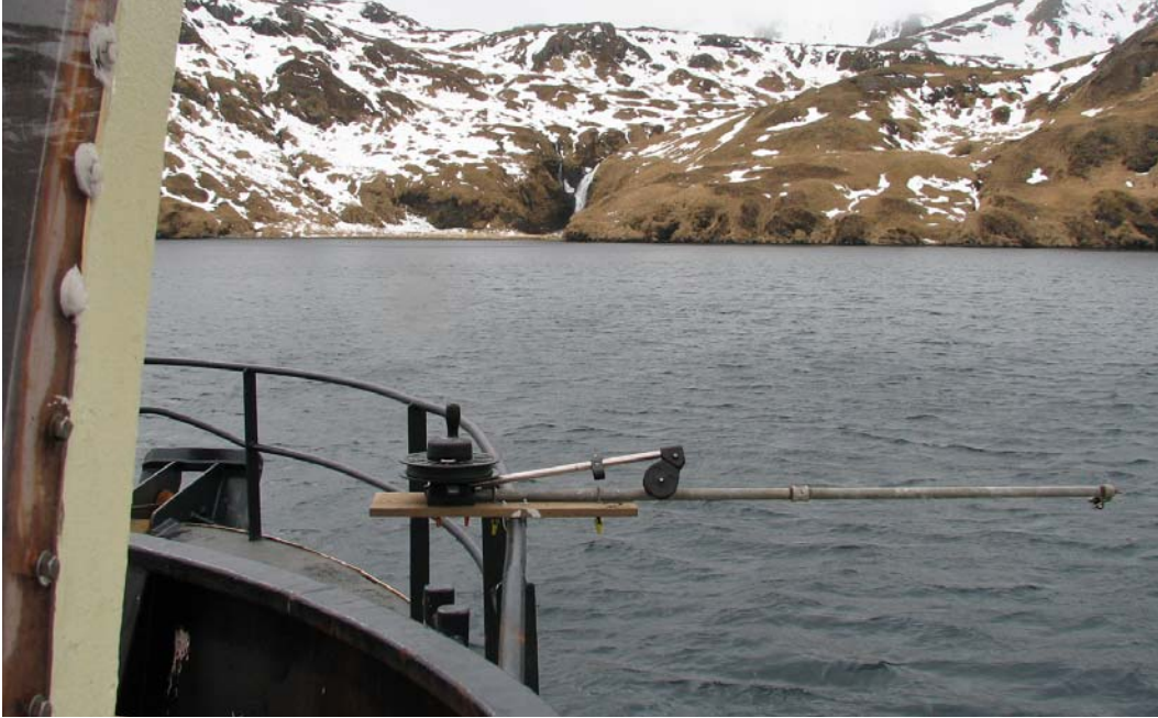
Figure 4.-- Starboard-bow downrigger setup for sphere calibration in Scabbard Bay near Adak Island, Alaska.
