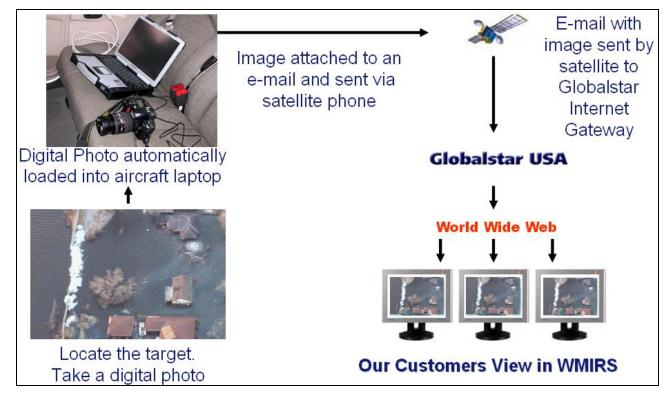
This is how SDIS works to provide near real-time imagery to customers from aboard CAP aircraft.
