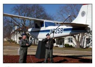
HSI operators collect the spectral signature of an aircraft on static display outside the CAP National Headquarters building at Maxwell AFB, Ala. The signature is then entered into the ARCHER airborne system database and used in a test to determine if the HSI equipment will pinpoint the static display plane from the air.
