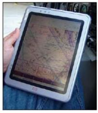
The ARCHER TRAC display shows the path flown by the aircraft and the exact ground area covered by the sensor as the flight progresses.
