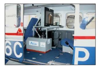
ARCHER system installed with custom-designed rack and protective hood in the Gippsland GA-8 Airvan. The third row of seats in the GA-8 is temporarily removed to install the ARCHER system when needed.
