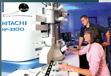
In Situ Microscopy – Transmission electron microscopy for in situ characterization studies evaluates the stability of battery electrode materials during rapid charge-discharge cycling.
