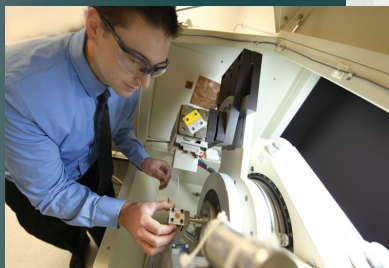
In Situ Fatigue Testing – An x-ray diffractometer is used to evaluate how battery materials change during charges and discharges.
