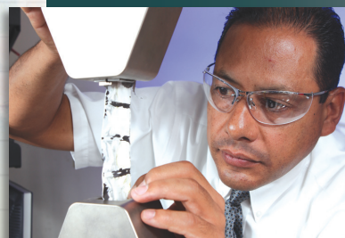
Mechanical Testing – A mechanical testing machine is used to characterize the stress-strain response of various battery materials.
