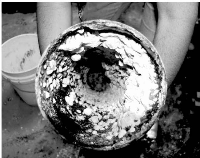
Figure 2 An 8" diameter cell with approximately 2" of \text{CaCO}_3 after 3 months operation.
