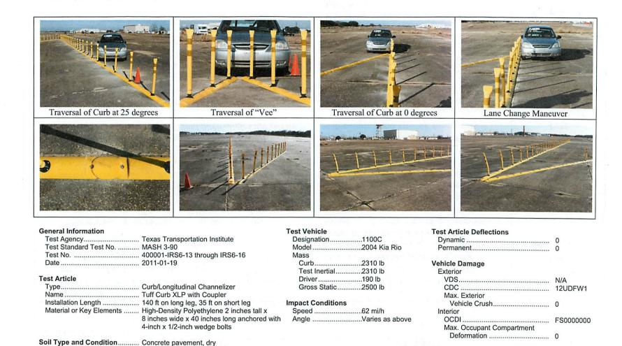
Figure 3. Summary of results for MASH test 3-90 on the Tuff Curb XLP with Coupler.
