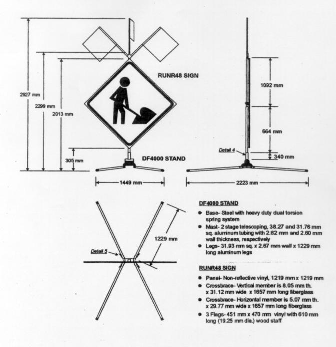
Figure 4. System Nos. 58 and 59 Sign Support Details, Test D-30
