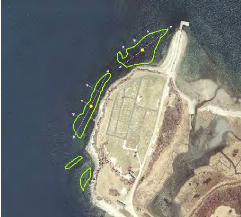
Figure 2. A strategy for field-mapping eelgrass beds was developed whereby GPS and video data were collected at the intersection of the arrows and polygons to determine the deepwater edge and extent of each eelgrass bed.
