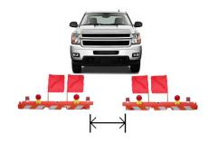
Space barricades such that a vehicle is unable to drive through gaps.
