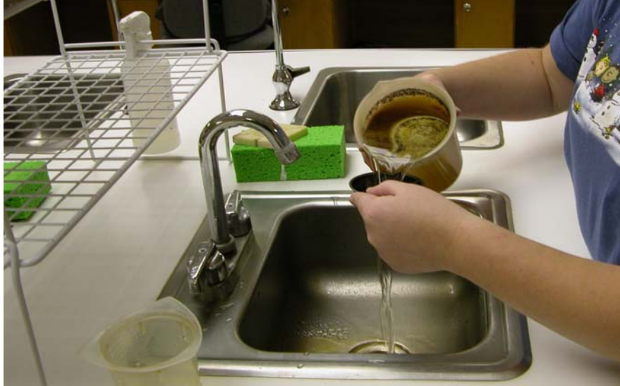
FIGURE 2-4-14 Pouring Sample from Beaker into Small #60 Sieve
