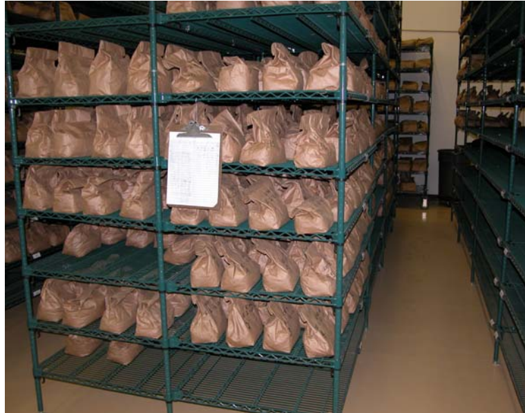
FIGURE 2-4-2 Soil Samples Drying in the Rack Room
