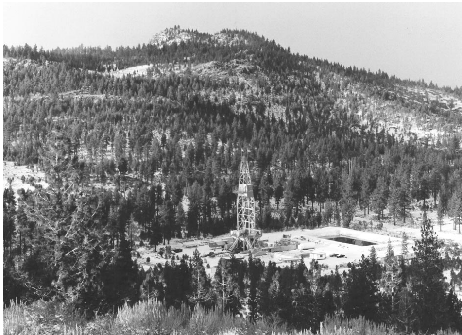
The Long Valley Exploratory Well is sited directly over the center of uplift on Long Valley Caldera's resurgent dome. Phase III drilling, begun in the summer and lasting through the fall of 1998, will extend the 7,200-foot-deep hole to between 11,500 and 13,000 feet, and greatly increase scientific knowledge of this restless volcano.
