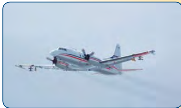
The Convair takes off on one of its 16 flight days from Fairbanks to Barrow, Alaska, during the month-long ISDAC field campaign. Both wings were heavily instrumented with cloud and aerosol probes.
