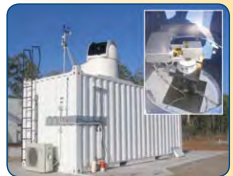
A camera, weather station, and sun tracker with a protective dome are located on the roof of the fully automated FTS mobile laboratory. Inside the shelter, the spectrometer receives the reflected solar beam from the sun tracker (inset), while the main computer system operates all the instruments and acquires the data.
