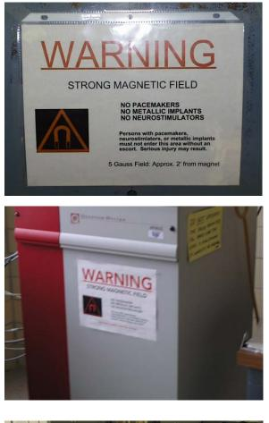
Picture 1. Sample magnetic field warning sign on laboratory door denoting 5 Gauss line.
