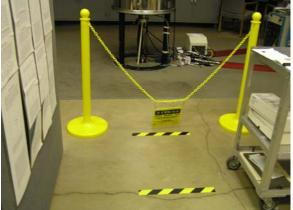
Picture 3. Warning sign on stanchions and floor markings denoting 5 and 10 Gauss lines.
