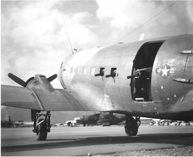
Side mounted 7.62mm mini-guns protrude from the door and windows of an AC-47 on the flight line at Nha Trang, AB, South Vietnam in 1967.
