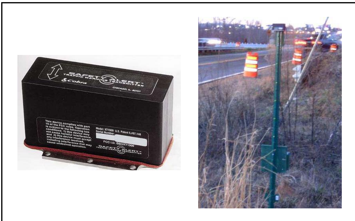
FIGURE 2.9 Cobra XT 1000 safety alert warning system attached to mounting structure in the field (Eckenrode et al. 2007)
