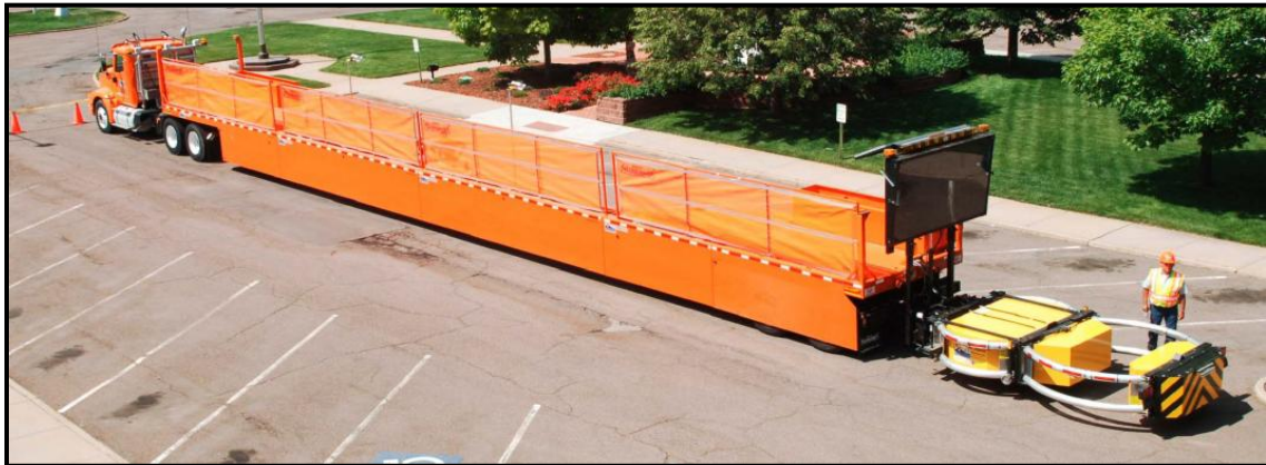
FIGURE 2.13 Mobile Barrier Trailer (MBT-1) System (Mobile Barriers LLC 2009)
