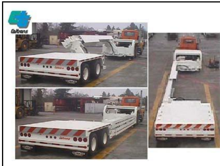
FIGURE 2.12 Balsi Beam mobile barrier system (California Department of Transportation)
