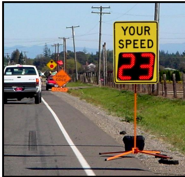
FIGURE 2.7 The installation of a portable speed monitoring display sign (Speed Check 2010)
