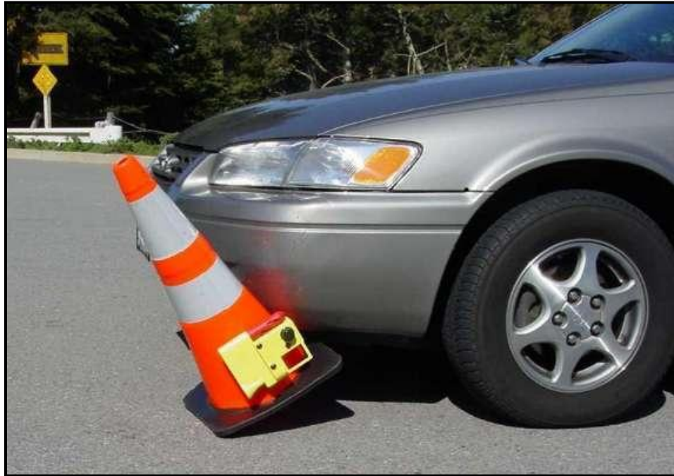
FIGURE 2.5 The installation of SonoBlaster Intrusion Alarms Devices (The Transpo Group 2010)
