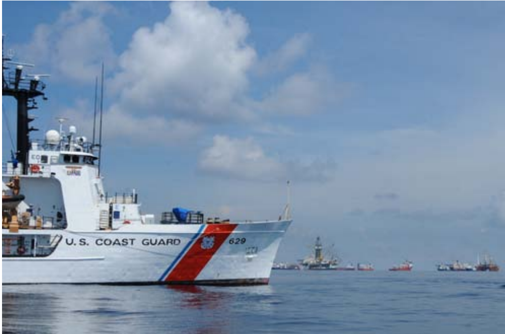
GULF OF MEXICO - The Coast Guard Cutter Decisive passes in front of the Q4000 while patrolling the area near the BP wellhead, August 3, 2010. The rig continues preparations to begin the "static kill", an operation in which heavy drilling mud and cement are slowly pumped into the wellhead to begin the process of killing it permanently. U.S. Coast Guard photograph by Petty Officer 1st Class Adam Eggers.
