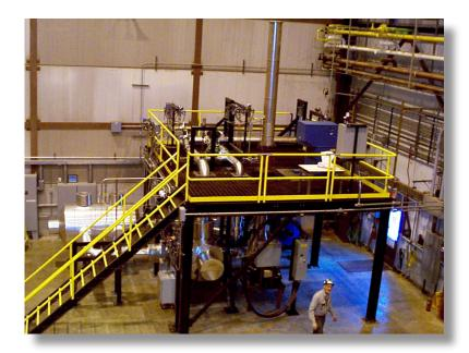
hybrid technology. NETL maintains a leadership position in this type of numerical simulation. As technical issues and potential benefits of the technology were identified, the need for hardware became apparent. An experimental test facility was designed and built at NETL's Morgantown site as a resource to researchers and industrial developers of hybrid systems. The facility is the only one of its kind anywhere in the world.
