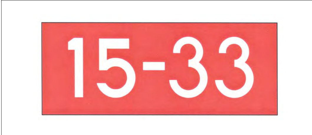
FIG 2-3-24 Runway Holding Position Sign
