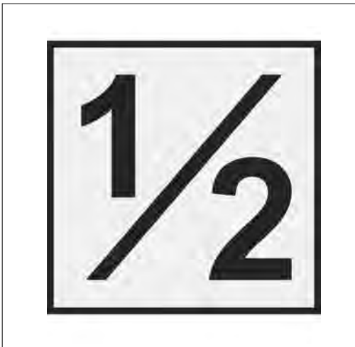
FIG 7-5-1 Typical Runway Half-way Sign
