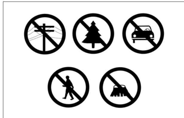
Landing Zone Hazards
