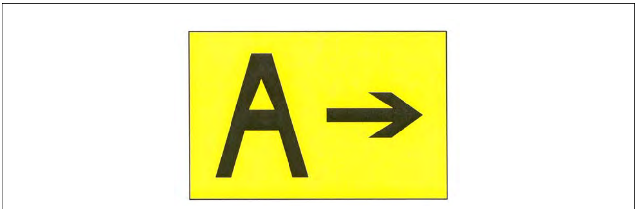
FIG 2-3-36 Direction Sign for Runway Exit
