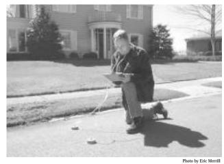
Shawn Menear, a graduate student in Technology Education at West Virginia University, uses geophones to listen for water main leaks. Similar to a doctor or nurse's stethoscope, geophones are an inexpensive leak detection device used by water utilities.
