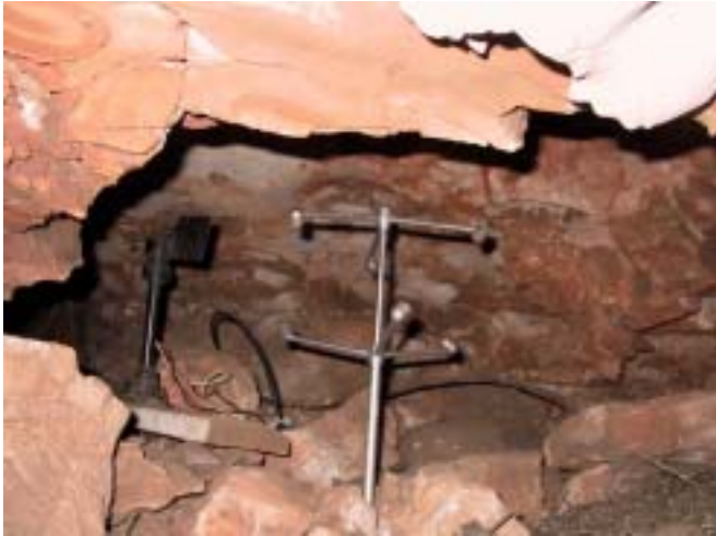
The Sonic Anemometer in the Natural Entrance. (NPS Photo by Rod Horrocks)
