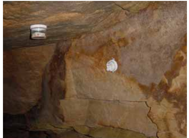
Caption: Temperatures were recorded using HOBO ® Pro H08 series dataloggers. Human disturbance events were measured using HOBO ® H06 Light event recorders.
