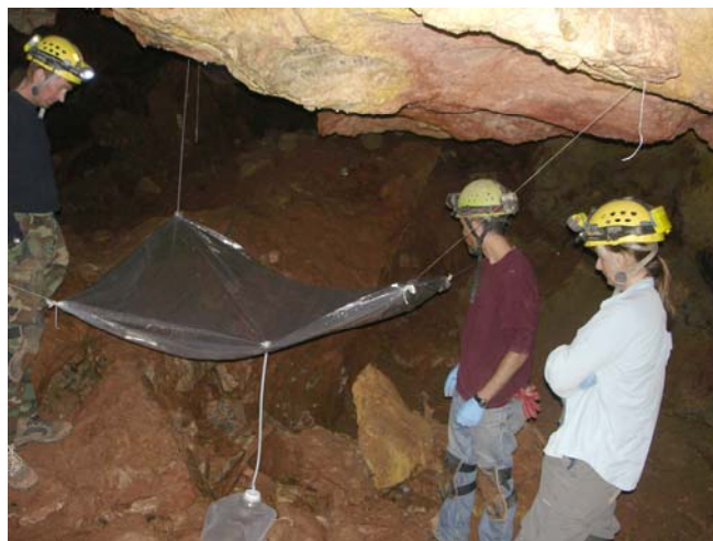
Marc Ohms, Andy Long, and Jennifer Back set up a drip collector in Room Draculum in Wind Cave.
