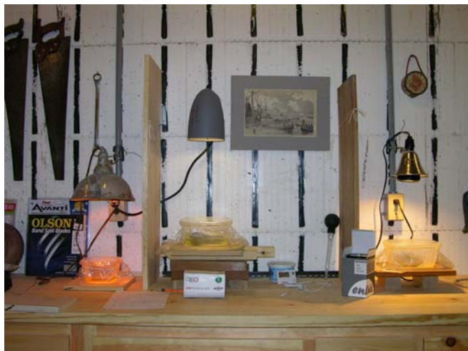
Fig. 1. Basement light test. Light on the left is the enLux W2050, the light in the middle is the Ledtronics XIW warm-white, and the light on the right is the Ledtronics 592 nm yellow LED lamp.
