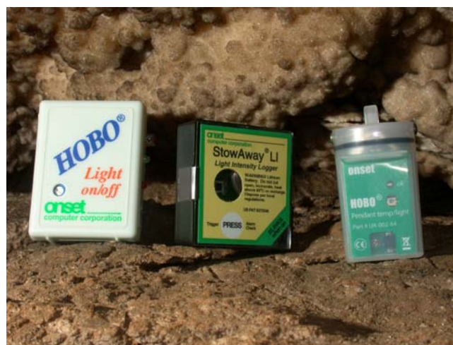
Fig. 1. HOBO H6 Light On/Off Logger, HOBO StowAway Light Intensity Data Logger, and HOBO Pendant Temperature and Light Intensity Data Logger being tested along the Mammoth Cave Wild Cave Tour route.
