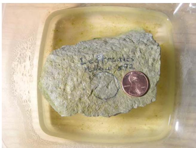
Fig. 3. Lampflora growth at 51 days under 592 nm yellow and W2050 white light at 145 foot candles. The results are similar, which is encouraging because the yellow LEDs have been in Frozen Niagara for 7 years and not grown any lampflora at a reasonable light intensity of about 4 foot candles.
