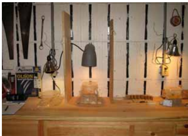
Figure 1. Latest bench test May 31-August 31, 2008. The enLux 2700 K lamp is at left, enLux 2050 lamp is in the middle, and the compact fluorescent is on the right.
