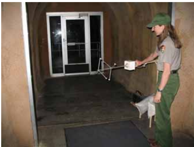
Rene Ohms holding an ultrasonic anemometer in the Upper Cave airlock in Jewel Cave (NPS photo).
