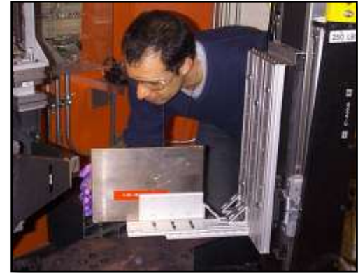
Mounting a plate test specimen for through thickness strain mapping at NRSF2
