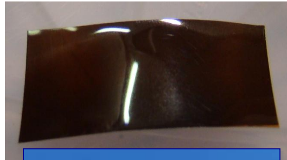
Low Cost Polycrystalline CdTe on Kapton Substrate
