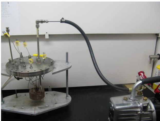
Static Test Chamber
