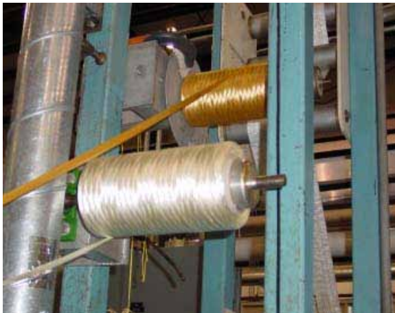
Figure 14. FISIFE precursor during processing (yellow). Conventional precursor is white.
