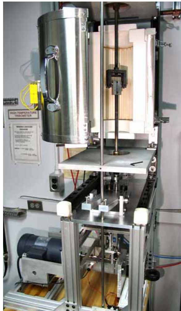
Figure 17. High temperature, repetitive impact testing machine with the furnace door open to reveal the specimen holders.
