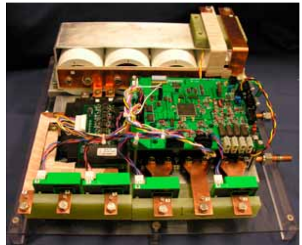
Figure 1: A 55 kW motor inverter and a 30 kW generator inverter with plug-in charging capability of 20 kW.
