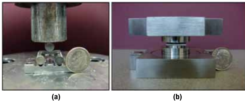
Figure 2: Uniaxial flexure (a) and biaxial flexure (b) testing of TE specimens provide needed strength data for TE device design.
