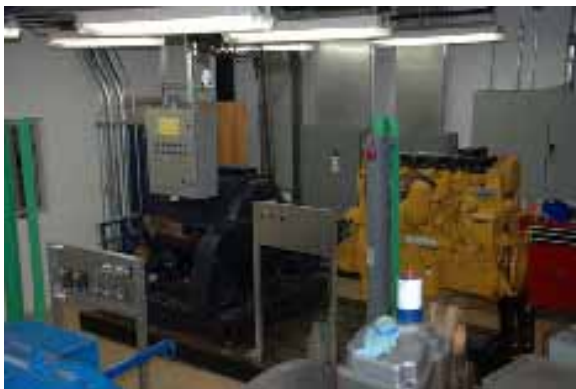
Figure 18. Photograph showing mounted Caterpillar engine and dynamometer in ORNL engine test cell. The engine will be used for testing advanced component designs and materials.
