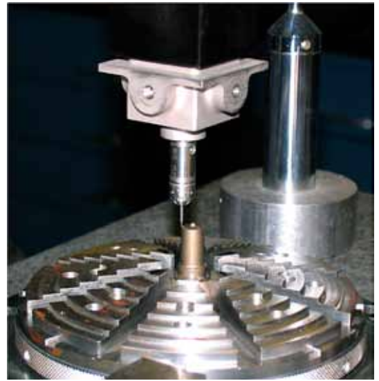
Figure 2: A high precision coordinate measuring machine provided dimensional data that were used to position injector tips for X-ray and neutron residual stress analyses.
