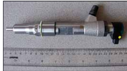
Figure 1: Piezoelectric actuated fuel injector used in Ford 6.4L Power Stroke diesel engine.
