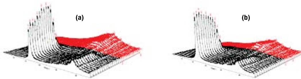
Figure 1: Morphological evolution as observed by online XRD during heat treatment of (a) as-spun polyacrylonitrile (PAN) and (b) radiation modified PAN fibers.
