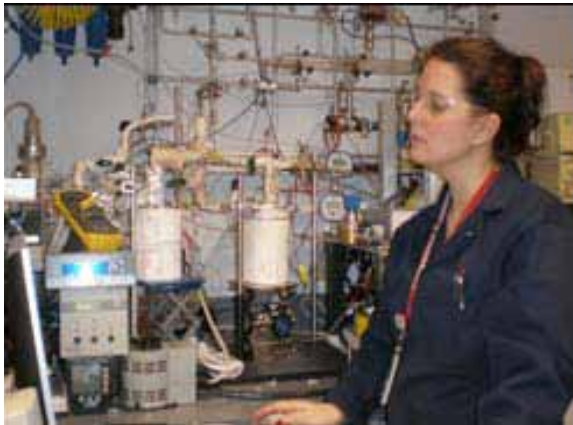
Figure 12. Microreactor experiment for soot oxidation studies.
