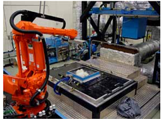
Figure 1: Robotic preforming machine at ORNL.
