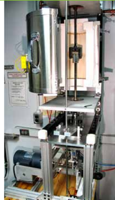
Figure 1: A high temperature, repetitive impact testing apparatus was designed and built for this project. It can accommodate simple coupons or actual exhaust valves.
