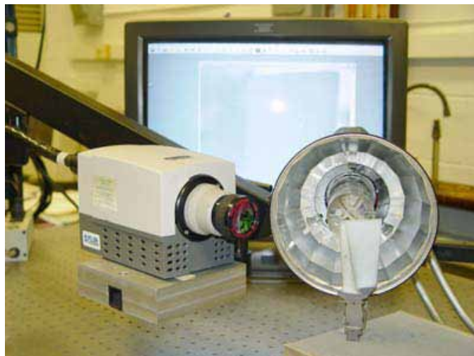
Figure 22. One-sided flash thermal imaging setup for testing of a turbine blade with TBC coating.
