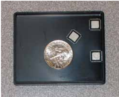
Figure 3: Three SOI gate driver ICs.
