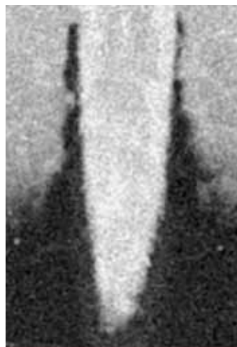
Figure 2: Elemental map of a scratch exposed to 850 °C shows that abrasion damage (center, brighter area) is oxygen rich.
