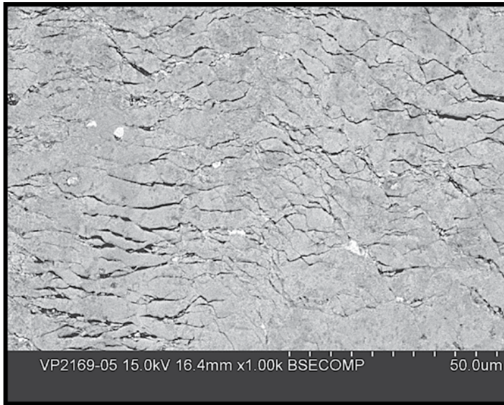
Figure 3: Back-scattered electron image of a densified, heterogeneous deposit of oxides of iron and chromium formed on a nickel alloy block after 20,000 impacts against a cobalt alloy pin at 750 °C in the HTRI apparatus (Figure 1).
