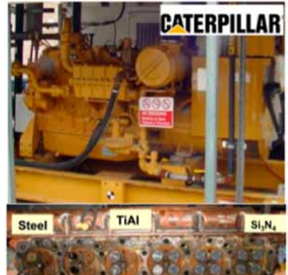
Figure 1: Photos showing Caterpillar G3406 natural gas engine and \text{Si}_3\text{N}_4 , TiAl, and steel valve locations in the engine.
