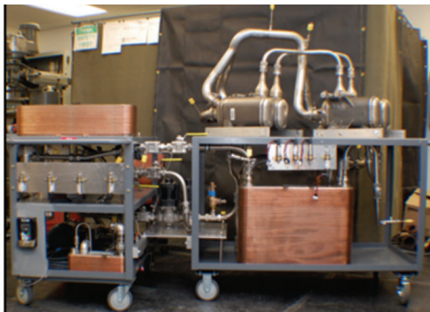
Organic Rankine cycle which is being used to convert exhaust heat to electrical power on a 1.9 L General Motors diesel engine.
