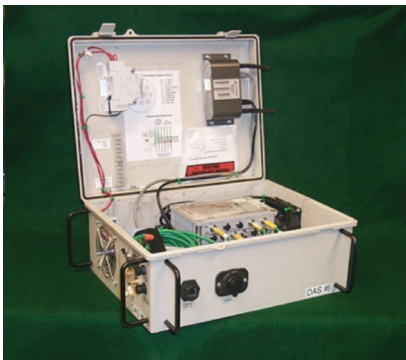
DAS that is installed in a truck cab.
