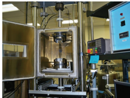
Tension-tension fatigue testing with the MTS Systems Corporation (MTS) test machine/oven chamber.
