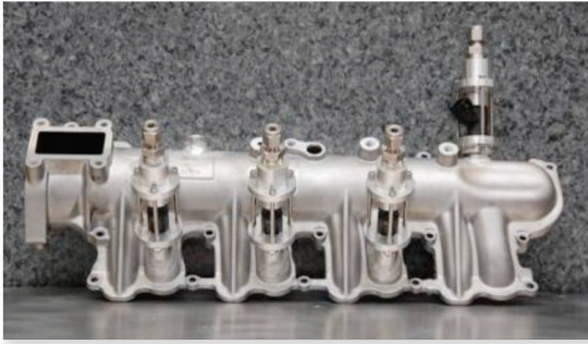
Modified intake manifold installed on engine (a) and with gasoline injectors installed (b).
