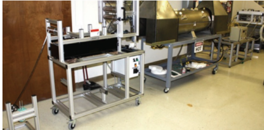
ORNL laboratory-scale experimental carbon fiber reinforced composite processing line: (a) continuous thermochemical surface treatment applicator; (b) continuous sizing line.
