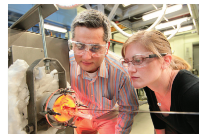
Carbon fiber tow exits the high temperature carbonization furnace.
