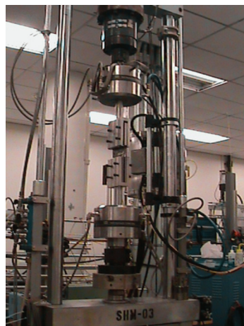
Cyclic torsion fatigue test with the MTS axial-torsional test machine.
