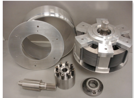
SR motor prototype parts.
