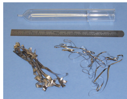
A typical melt-spinning crucible and two melt-spun ribbons of \text{Hf}_2\text{Co}_{11} -based hard ferromagnetic materials.
