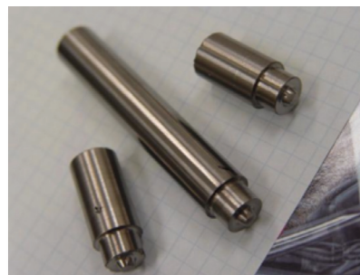
Stir tools made from metal matrix composites.
