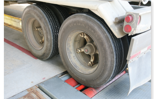
Performance-based brake testing technology provides a safe, accurate, and objective assessment of a vehicle's brake force and overall brake performance.
