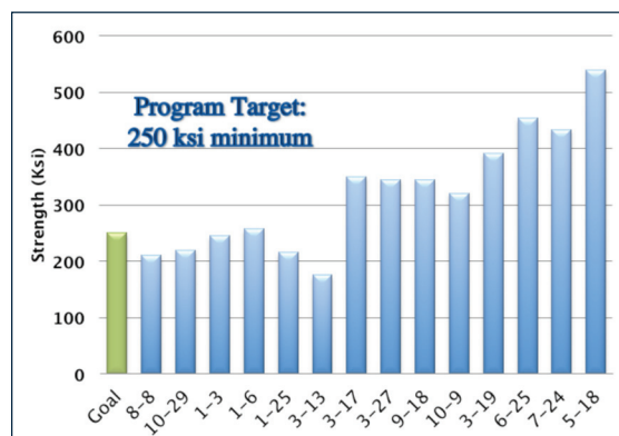
Improvement in fiber strength during the project.
