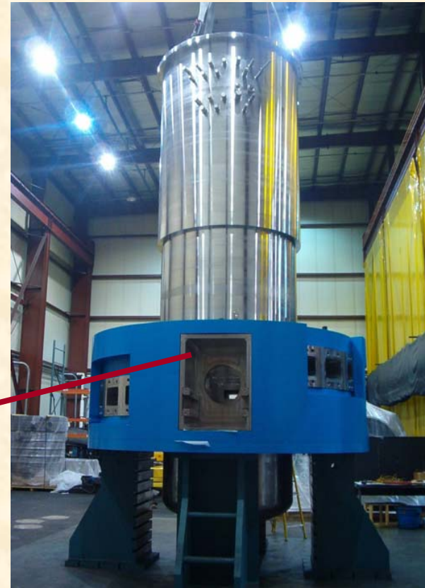
Core Vessel and Shielding
