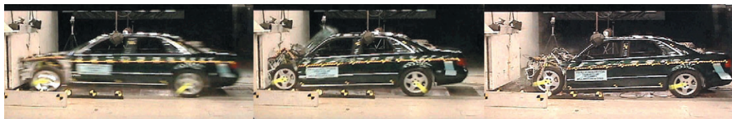
Images of an all-aluminum Audi A8 car during an actual crash test. The car hit a rigid barrier at 35 miles per hour. The crash data are used to help ORNL researchers improve their car-crash computer models.
