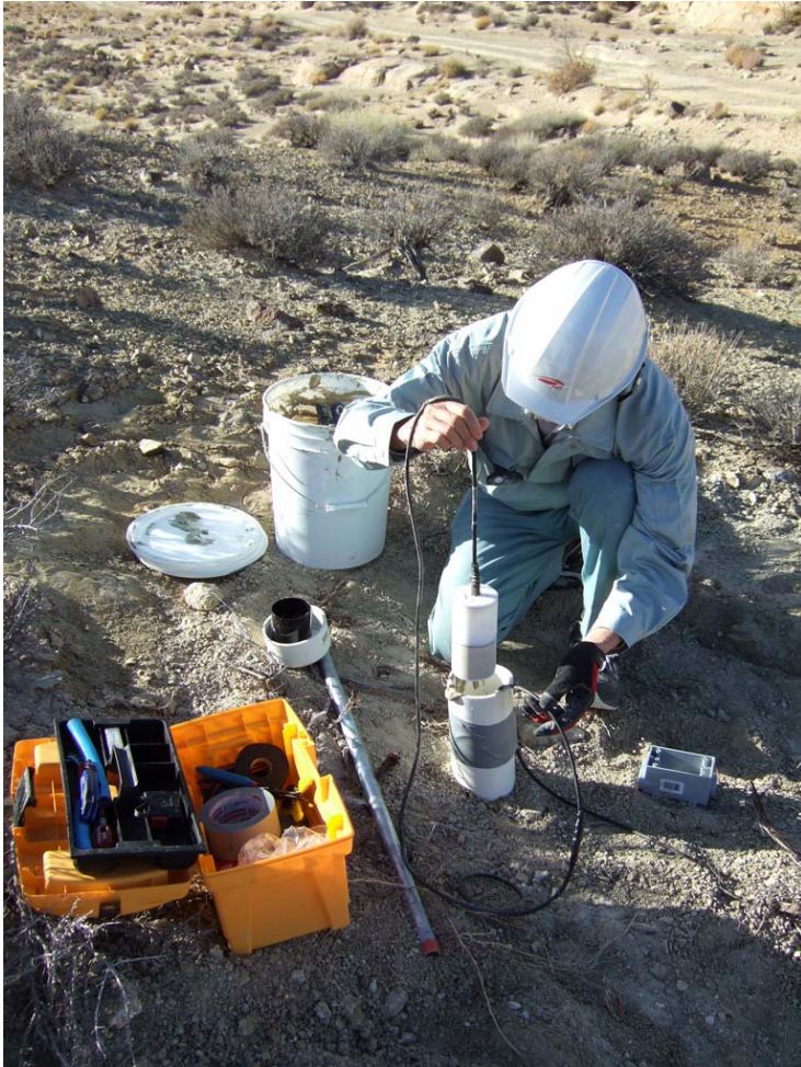
Installation of Ag-AgCl electrode
