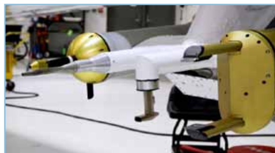
The high-volume precipitation spectrometer (front) measures the number and size of precipitation particles, including snowflakes, from 150 microns to 1.92 centimeters in size. This is the only aircraft research instrument of its kind that provides complete digital images of precipitation particles up to nearly 2 centimeters in size.
