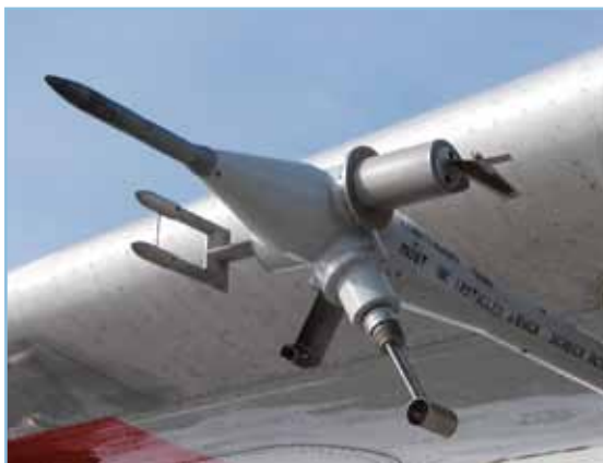
This probe "boom" on the wing of a Canadian National Research Council's Convair 580 includes a variety of instruments to measure total water content, liquid water content, temperature, and pressure.
