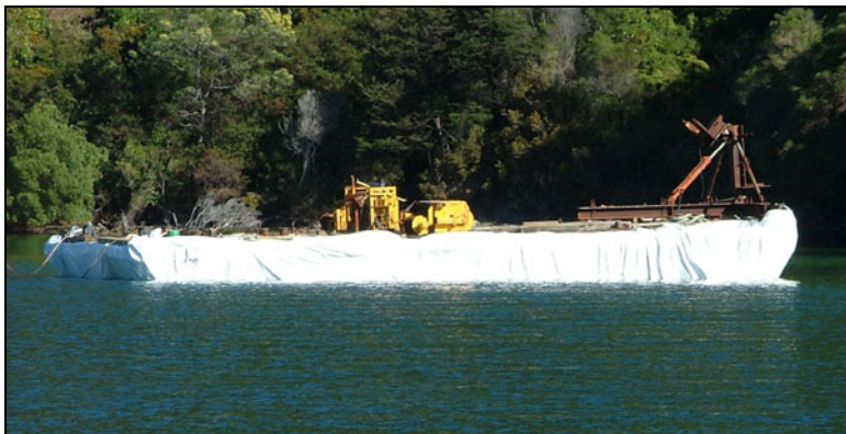
Figure 9. Various vessel types affected with D. vexillum were treated using a set-n-forget in situ plastic encapsulation technique.
