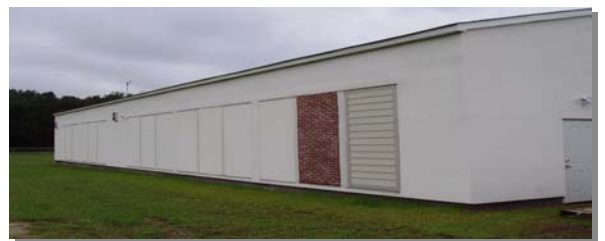
The EIFS Industry Members Association underwrote the cost of a natural exposure test facility in Charleston that can test 15 different wall systems side by side.
