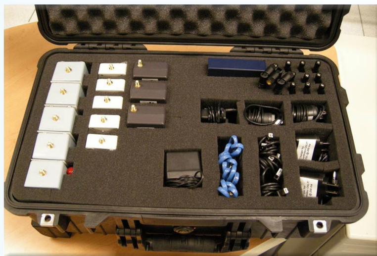
ORNL wireless sensor suitcase used to demonstrate wireless capability in the Alcoa manufacturing plant.
