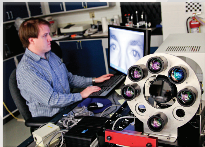
Chris Boehnen demonstrates an ORNL-developed video imaging device that can follow an individual's movement, capturing 30 iris images per second from a distance of 25 feet.
