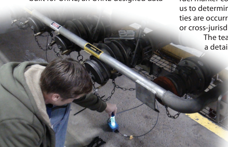
MSSSED's Duncan Earl calibrates fuel marker sensor using a calibration vial filled with #2 diesel fuel and fuel marker dye.
