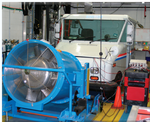
U.S. Postal Service electric vehicle on dynamometer
