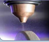
Direct Metal Deposition uses inert gas to spray powder into a melt pool created by a high-power laser beam.
