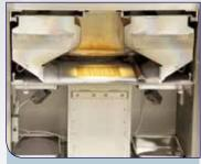
Metal Powder Bed Consolidation uses a high-power electron or laser beam to create a site-specific melt pool in a bed of metal powder.
