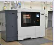
Polymer Extrusion uses a heated nozzle to deposit small beads of thermoplastic material into a two-dimensional pattern.
