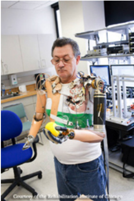
A patient wears a six-motor "bionic arm" — a neuro-controlled prosthetic arm — developed by researchers at the Rehabilitation Institute of Chicago and the Johns Hopkins Applied Physics Laboratory.
