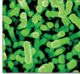
Assembled using viruses, these nanowires are coated in silicon, which has a higher energy density than graphite, the material typically used in battery electrodes.
