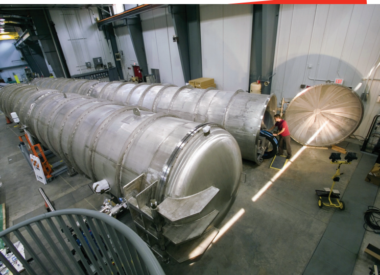
HFIR Instrument Support Manager working on the General Purpose SANS Instrument in the Cold Guide Hall
