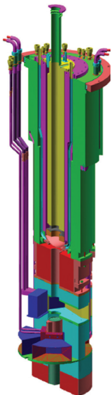
The advanced target-moderator assembly at the Lujan
