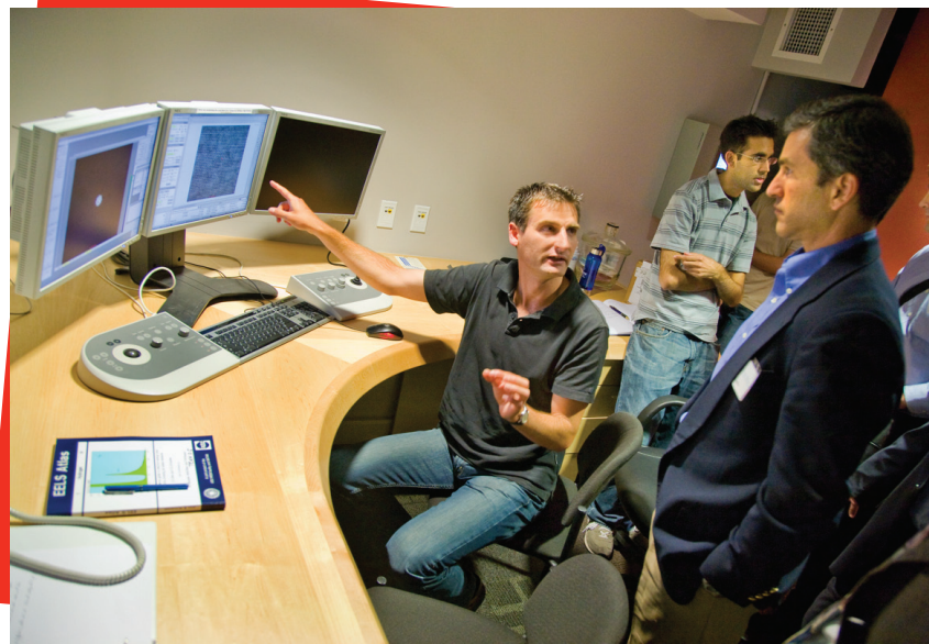
TEAM 0.5 is controlled from a remote workstation and operates as a user instrument.
