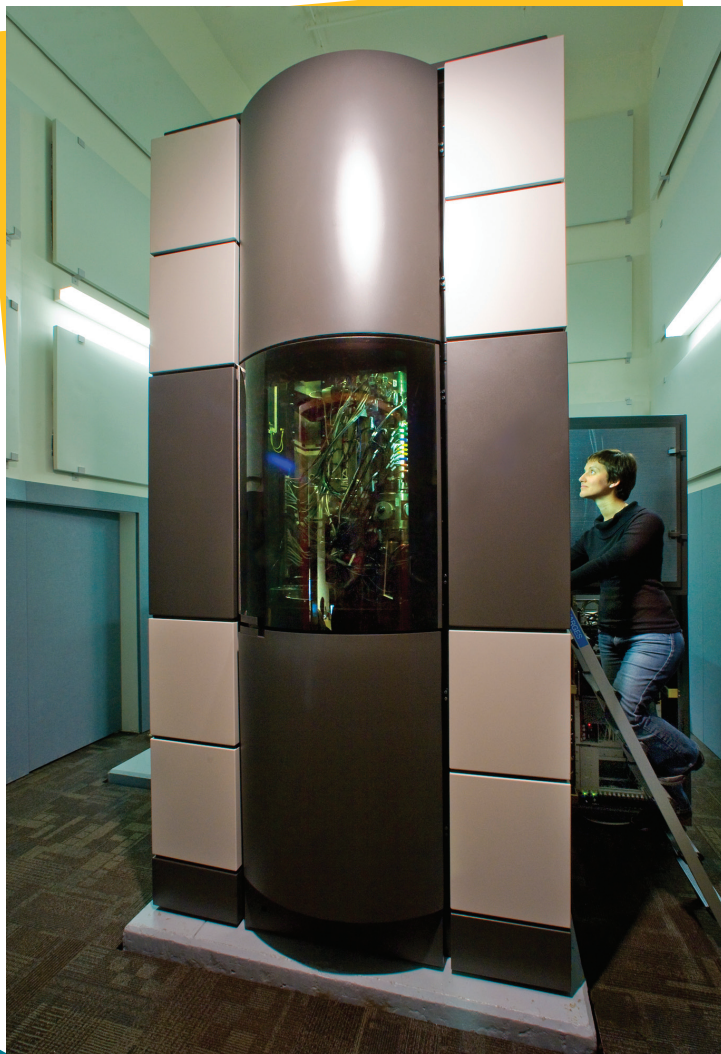
The world-leading monochromated, aberration-corrected TEAM 0.5 microscope is capable of half-Angstrom imaging in both, broad-beam and scanning-probe modes of operation.
