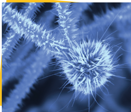
Cu-TCNQ nanowires on ZnO nanowires. Here TCNQ is the common abbreviation for 7,7,8,8-tetracyanoquinodimethane, an organometallic semiconductor charge transfer material. (Courtesy of Kai Xiao, CNMS, Oak Ridge National Laboratory.)
