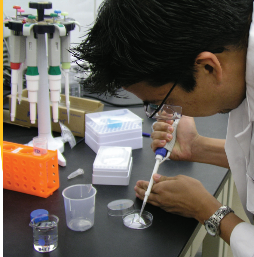
Preparing a slide of quantum dot attached microtubules for an atomic force microscopy experiment.
