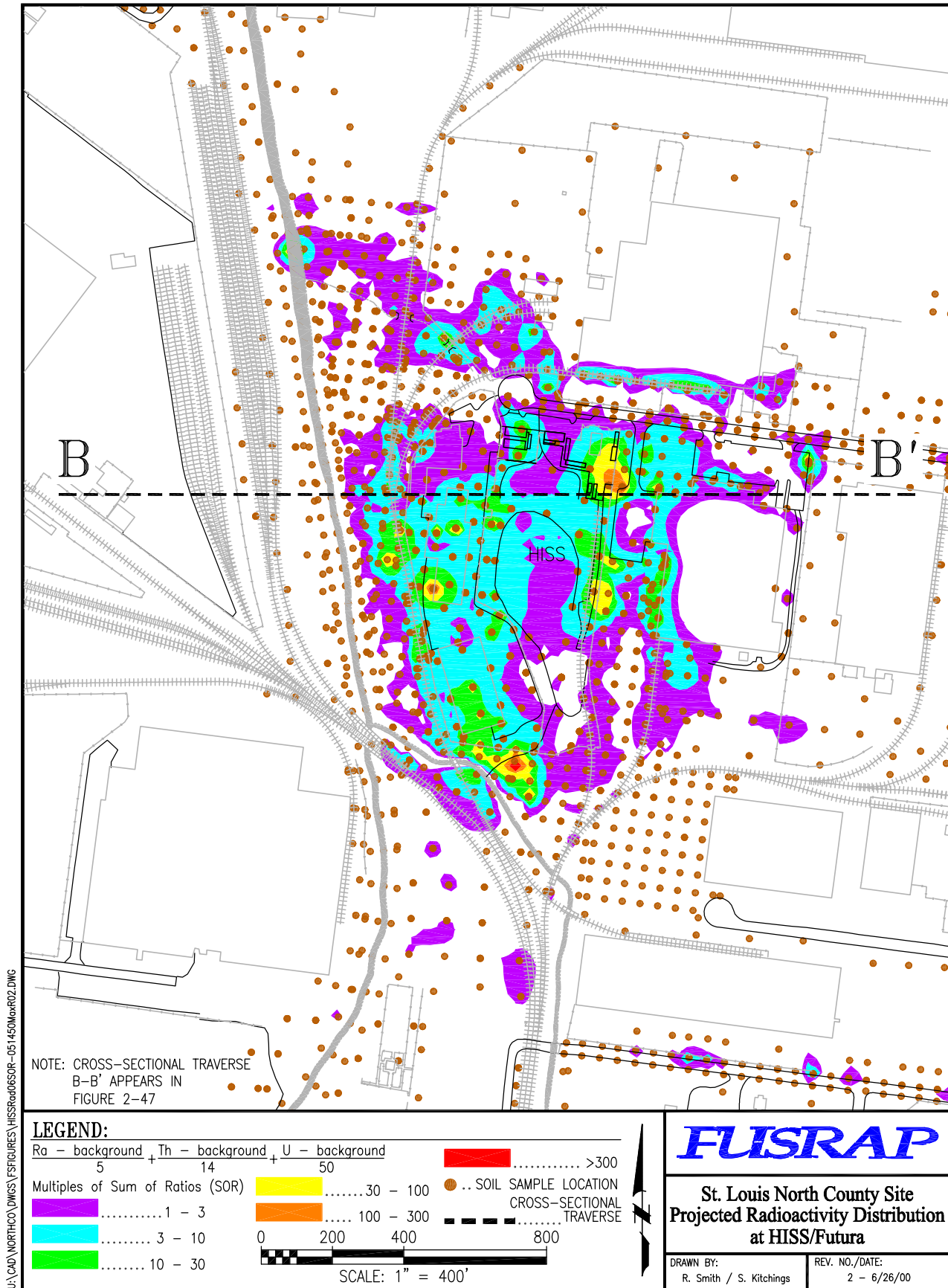
Figure 2-46. Projected Radioactivity Exceeding 5 pCi/g of Radium-226, 14 pCi/g of Thorium-230, 50 pCi/g of Uranium-238 or Combination Such That Sum of Ratio = 1 at HISS/Futura
