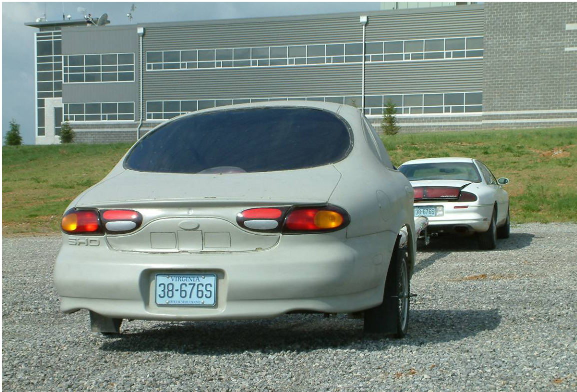
Figure 9. Rear of the surrogate vehicle with the imminent-warning lighting panels closed.
