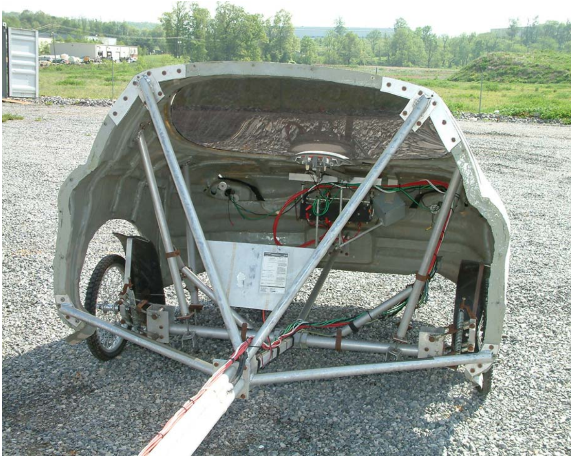
Figure 12. The interior of the surrogate vehicle shell. Note that the front curtains (fairings) have been temporarily removed for this photo.
