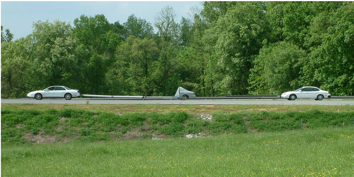
Figure 7. Towing/surrogate vehicle combination shown with the following vehicle. Note that the following vehicle is closer than during the actual experiment.
