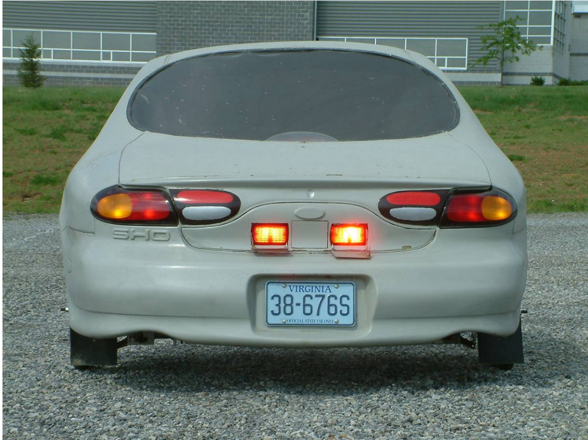
Figure 11. The IAP imminent-warning lighting signal with its snap-down panels open. (Lamp output was subjectively “redder” than it appears in this figure.)
