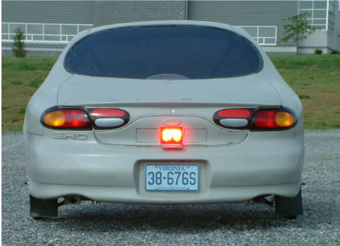
Figure 10. The TCL imminent-warning lighting signal with its snap-down panel open. (Lamp output was subjectively “redder” than it appears in this figure.)
