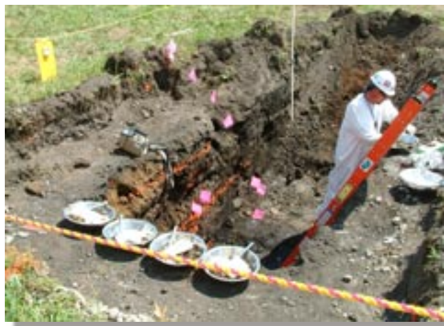
Collecting PDI samples from test pits allows sampling crews to better investigate any geological features of interest.
