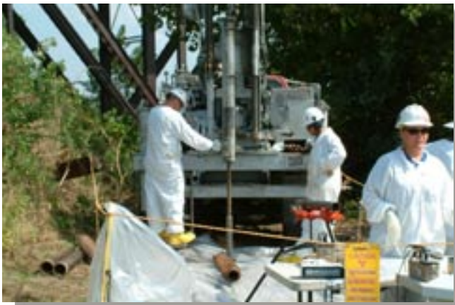
Drill crew collecting soil samples on the City of Venice, Illinois Vicinity Property DT-11 south of the McKinley Bridge to delineate the extent of contamination.
