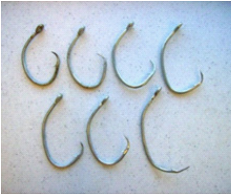
Hooks that retained bluefin tuna during the experiment: traditional hooks in the top row and weak hooks in the bottom.
