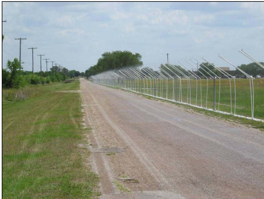
Figure 35. Test Course with Rain Tunnel.
