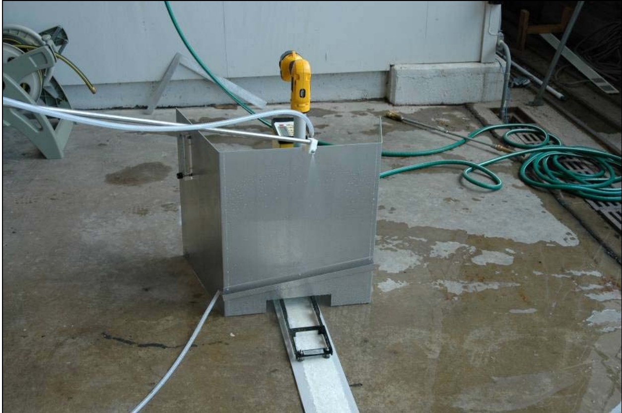
Figure 30. Wet Retroreflectivity Observation Method.
