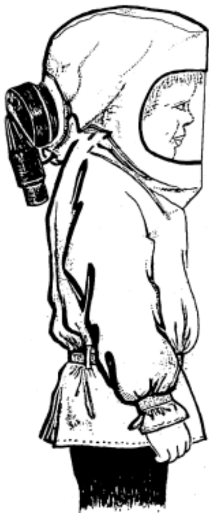
Fig. C.2. Protective jacket and hood for children. See Trelleborg AB, Protective Jacket (type 36) , manufacturer's brochure, S-23181, Protective Products Division, Trelleborg, Sweden, 1987; Forsheda Group, Forsheda, A Worldwide Group of Polymer Companies , manufacturer's brochure, 33012, Forsheda AB, Forsheda, Sweden, 1987.
